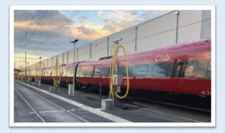
CET systems now integrating automatic winch for recovering flexible hoses and improving anti-spillage system. Clean and safer as never before.
