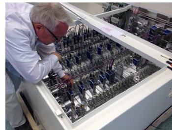
Gas handling system for an epitaxy reactor.
